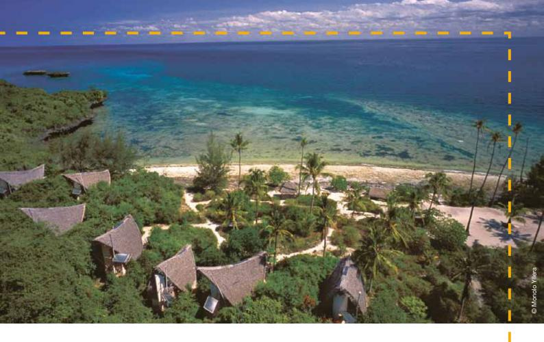
from Zanzibar Island and brought across by sailing dhow on a high tide to avoid damage to the coral reef. Casuarina poles were used for the main structural components, formed into shell-like roof shapes to facilitate rainwater collection and covered with palm thatch (*makuti*).
