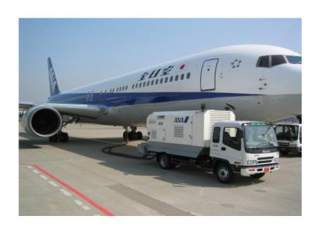
Water truck for drinking water is pumped into the aircraft's tank
